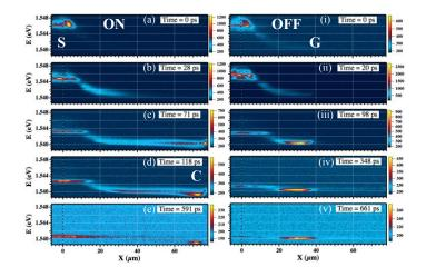
Figure 2. (a-e)/(i-v) Polariton emission in energy vs. position maps for the ON/OFF transistor state. The snapshots are taken at the times shown. The intensity is coded in a false color scale
