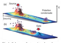
Fig.1. Scheme of a transistor based on a polariton condensate in a microcavity ridge (a) without and (b) with the gate.
